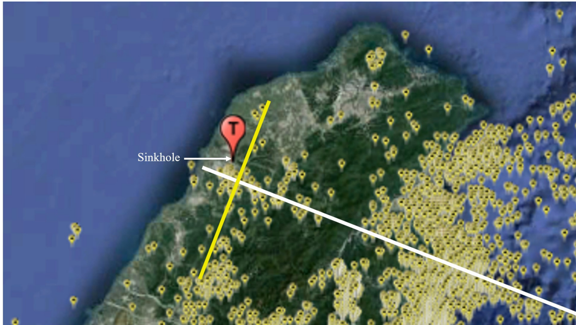
Figure 16. Identification of shear bands existing in the vicinity of Zhubei, Taiwan using the historical epicenter distribution map (Google Earth, 2023; Central Weather Bureau, 2016).
