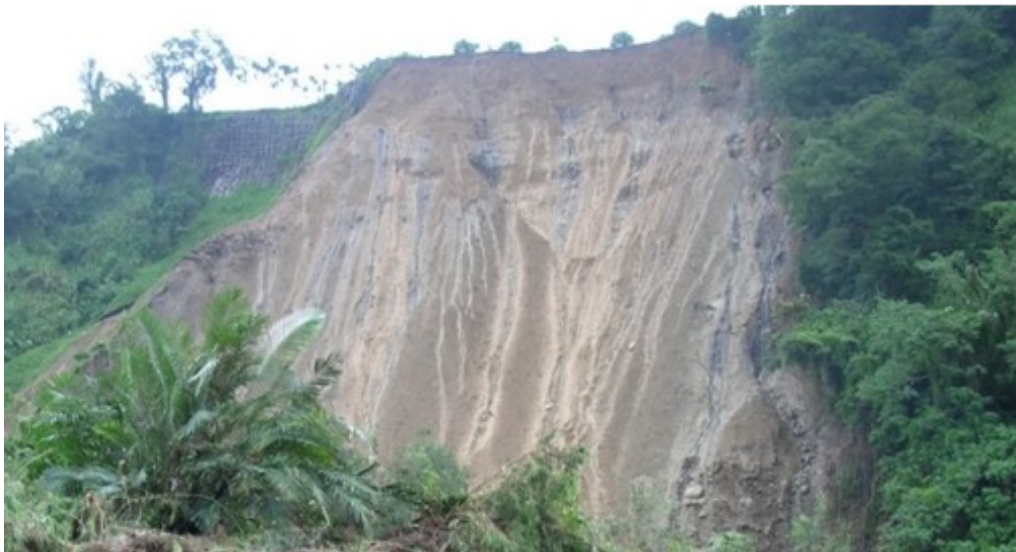
Figure 13. Groundwater entraining soil particles flowing out from a water outlet of the shear band outcrops (Nantou, Taiwan).
